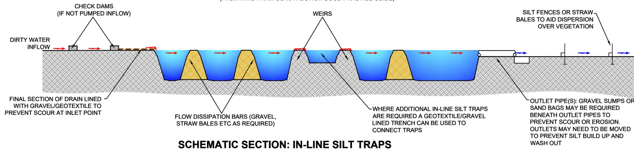
**SCHEMATIC SECTION: IN-LINE SILT TRAPS**
