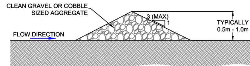
**IN CHANNEL ROCK CHECK DAM SECTION**
