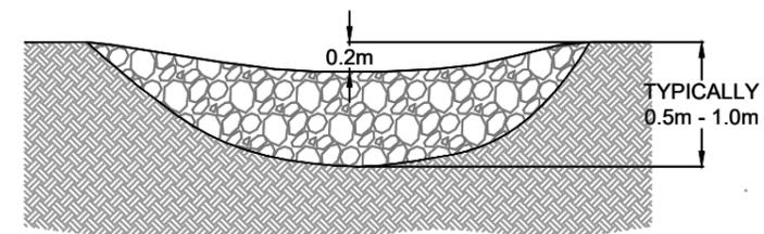
**IN CHANNEL ROCK CHECK DAM ELEVATION**
