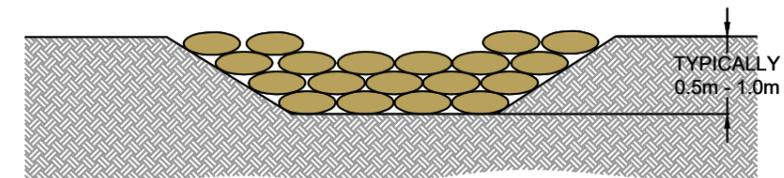
**IN CHANNEL SAND BAG CHECK DAM SECTION**
